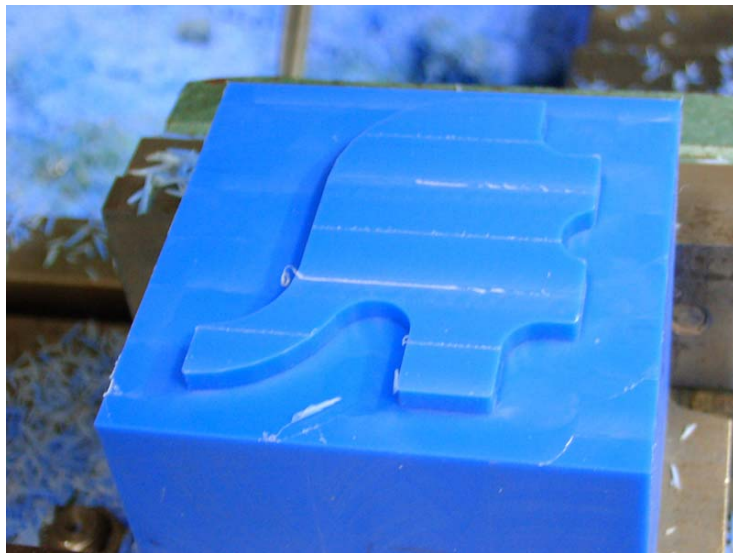
Fig 13. End of roughing process
